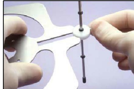
2. Attach disposable Index Tray to Analyzer bow by aligning protruding pins on Index Tray into the holes in the bite fork section of the Analyzer bow. Seat Index Tray all the way flat onto Analyzer bow.
